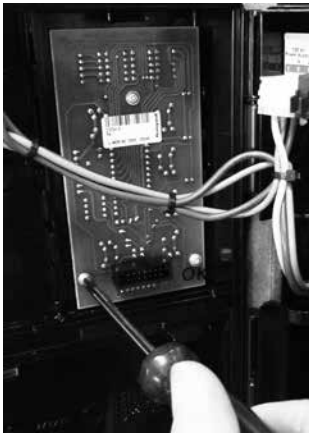
Replacing PCB fig. 3
